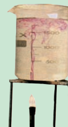
Fig 5.27 - Convection currents in a liquid
