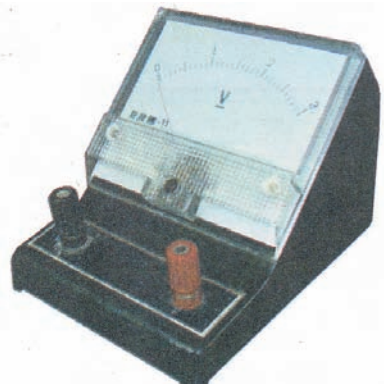
Fig 5.56 - Ammeter and Voltmeter used in laboratories
