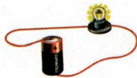
Fig. 5.49 - How to light a bulb using an electric cell
