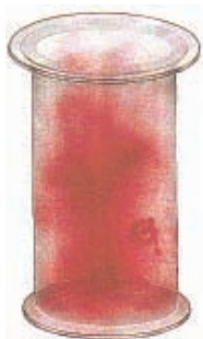
Fig.5.2 - A gas (iodine vapour) takes the volume of the vessel
