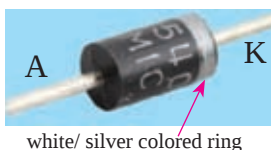
Figure 11.11 - General outward appearance of a junction diode
